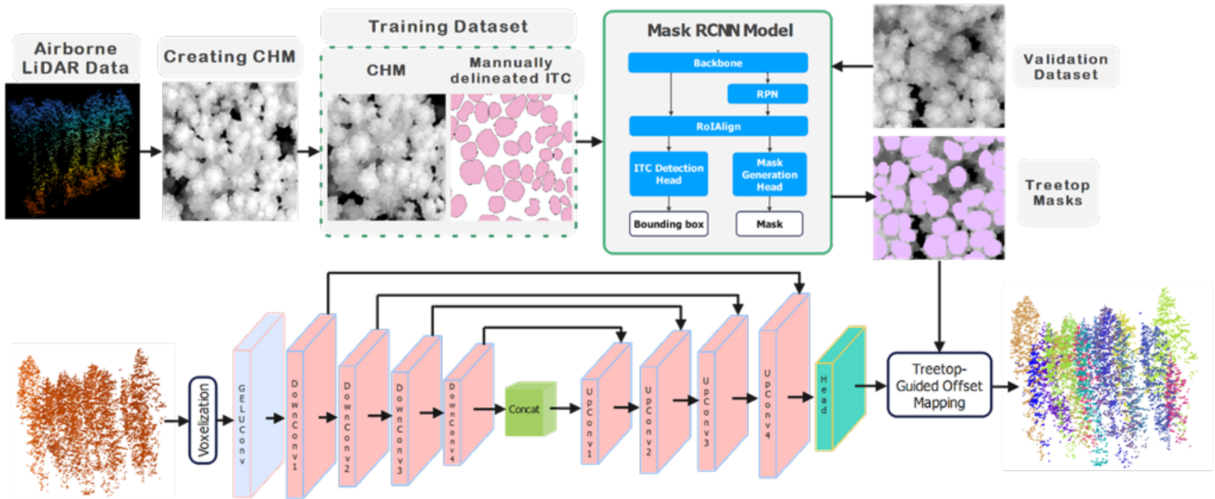
Figure 4. Workflow for the two-stage deep learning network combining Mask R-CNN and 3D U-Net.
