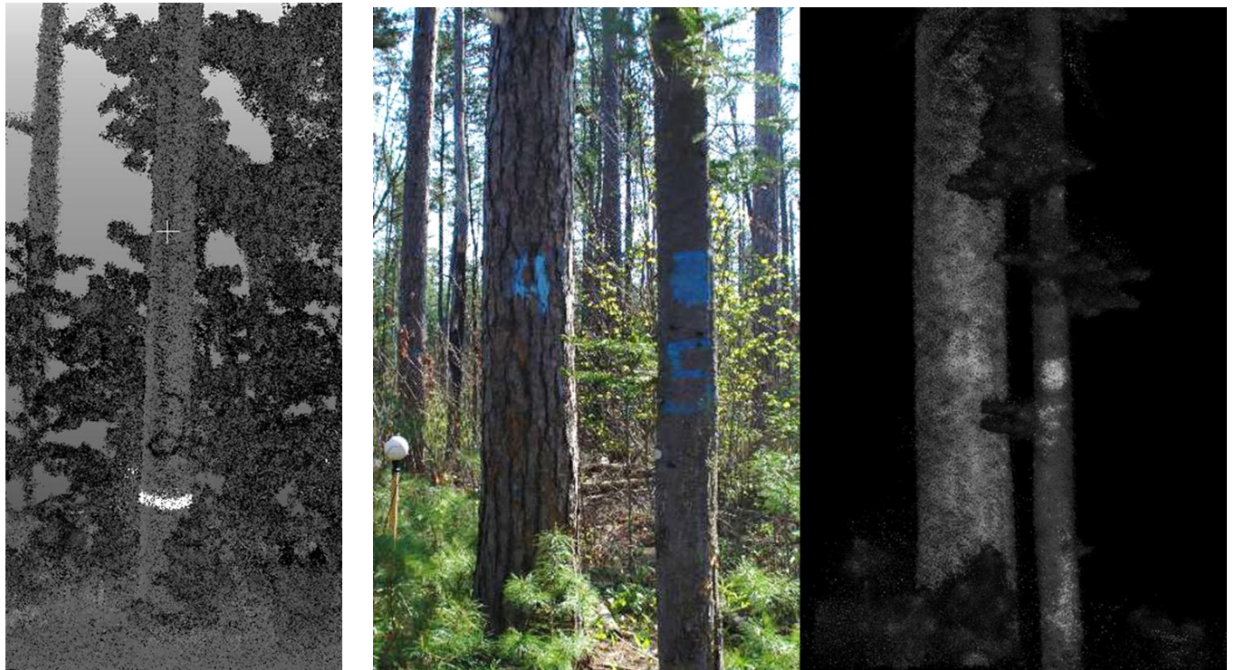
Figure 21. 3M reflective tape showed up well in the intensity field of tree scans. Fresh black or blue painted tree numbers showed up reasonably well in some conditions but depended on tree size, bark condition and age of paint.
