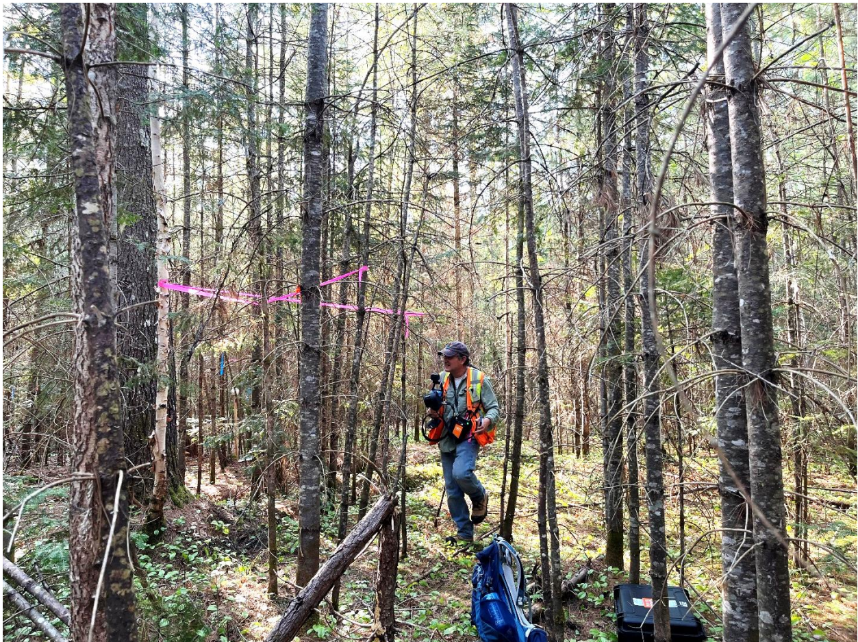
Scanning plot PRF002 with the Faro Orbis.
