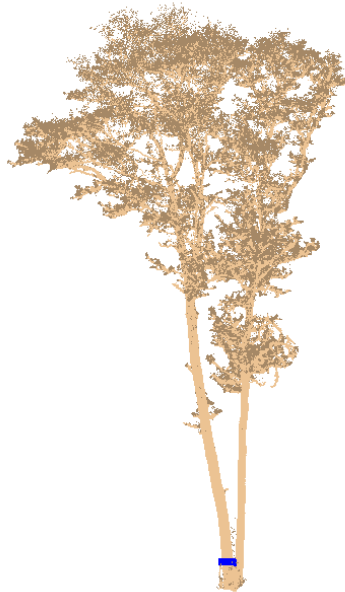
Figure 24. Example of an r-lidar pipeline segmented tree (DBHs of both stems >35 cm) that is forked below breast height. This tree should be segmented into two separate trees but is segmented as one, with only a single DBH fit to one stem.
