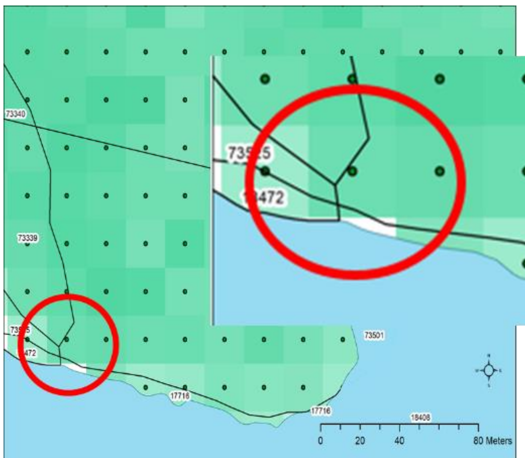
Figure 29 - Example of a raster pixel being bisected into 4 by polygon boundaries with only one polygon including the centroid value.
